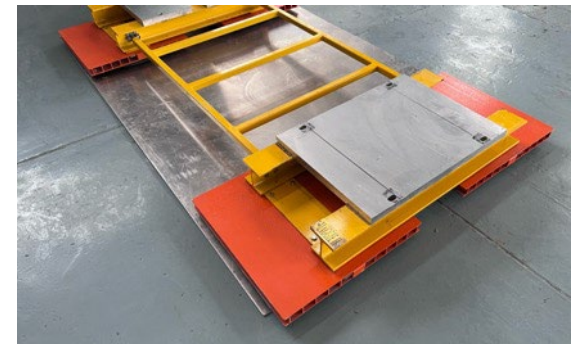
The aircart Maggie II used to move steel beams doe DUNE
