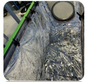
Thermal shield interior MLI installed.
