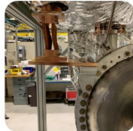
Cryocooler link shown connected to cooling rings on cavity
