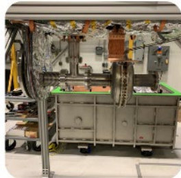
Cavity string with cryocooler link attached.
