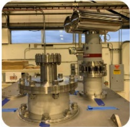
Top plate shown, with cryocooler head and mock coupler.
