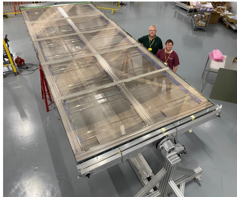
APAs for Module 0 ProtoDUNE being tested at Daresbury Laboratory, UK. One 2.3m x 6.3m APA is shown; UK to provide 130 APAs.
