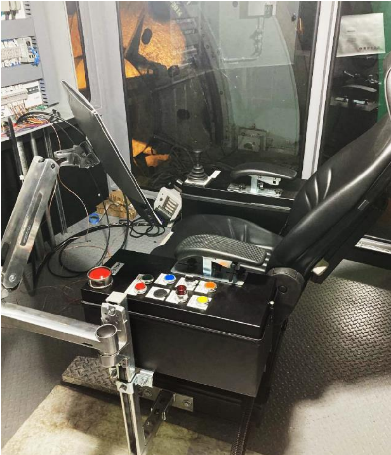
New Hoist Control Center with Flat Screen Monitors and Joystick Controls
